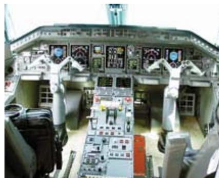
The Legacy flight deck is built around a five-screen Honeywell Primus 1000 system.
