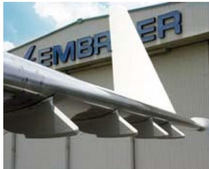
Vortillons beneath the leading edge of the wings help improve stability, especially because of the yaw produced by the winglets.
