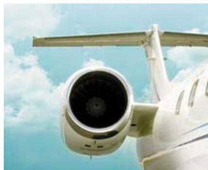
The Legacy is powered by a pair of Rolls-Royce AE3007-AE1 turbofans.
